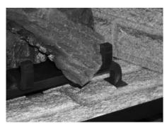
Place the bottom left front edge of Log 02-55 against the rear bracket on the burner tray and rest the log on the cutout onL o g 02-53.
